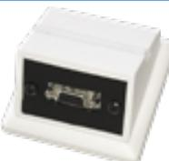
Flush mount box for DIGISystem desktop call stations with a lockable 9-pin Sub-D socket connector including an EMI/RFI filter. Quick coupling with spring clips. The outlet may be configured either vertically or at a 30° tilt. Pure white and complete with GIRA system 55-fitting uniframe. Intended for use with surface mount housing (Part No. 581329).
