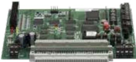
The serial essernet interface can be used as a gateway to link remote computers that support the ESSER by Honeywell data protocol (EDP). The EDP version (bidirectional) with remote control options e.g. for the connection to a Building Management System (BMS). The unit includes a slot for an essernet module and is therefore a fully functional unit within the short circuit and open circuit resistant essernet.
