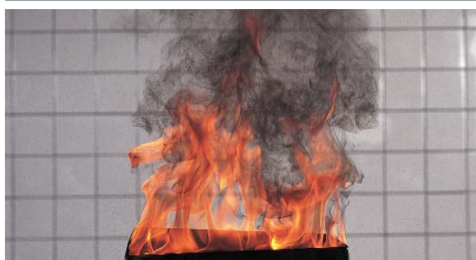
Test fire 5: liquid fire (n-heptane)
