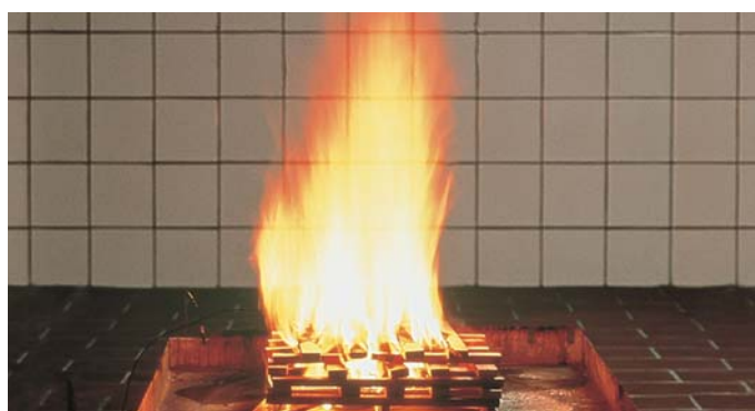
Test fire 1: cellulose open fire (wood)
