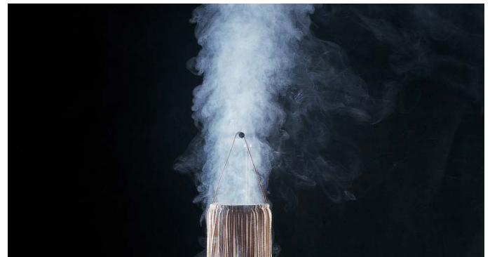
Test fire 3: glowing smoldering fire (cotton)
